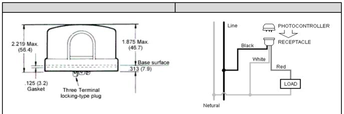
**Install the photocontroller with the Photocell facing the NORTH direction as indicated on the top of the photocontroller.** Adjust the receptacle position if necessary.
